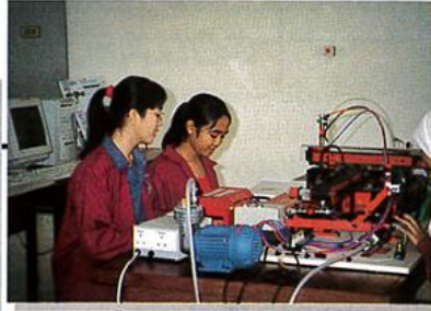
Control Lab:- The application of PLC to control processes in an assembly line
