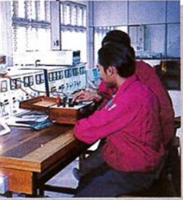
Measurement lab- Wheatstone bridge trainer - an experiment carries out to measure unknown resistance
